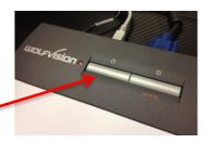
You can zoom in and out using the thumb wheel on the head unit.
